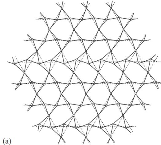
Figure 2: (Replotted from [3]) The dotted lines are the undeformed standard kagome lattice; the solid lines are the non-trivial Guest-Hutchinson mode for the standard kagome lattice. In the deformed lattice, there are some vertices still stay at the same position, while the others move with different displacements. And the GH mode is periodic with a different periodicity compared to the non-deformed standard kagome lattice.
