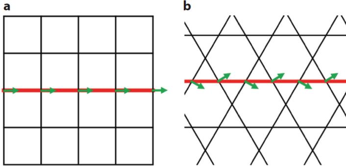
Figure 1: (Replotted from [5]) Figure a and b both have each vertex connecting 4 bars, thus they are Maxwell lattices. Figure a is a square lattice. It is non-rigid and we can deform every vertex with a same amount in the horizontal direction. Figure b is a standard kagome lattice. It is also non-rigid with a floppy mode shown in green arrows.
