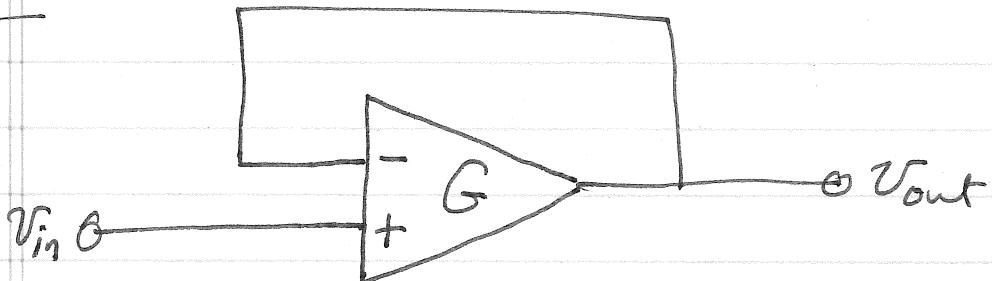
$$V_{out} = G(V_{in} - V_{out})$$
