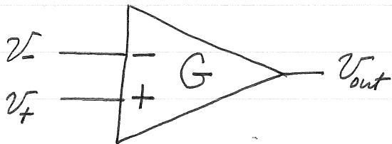
$$V_{out} = G(V_+ - V_-)$$
